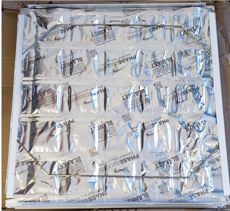
Figure 3. Macro-encapsulated PCM inside aluminum, captured by thin metal rod frame
