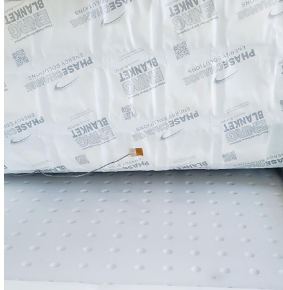
Figure 5. Self-adhesive thermocouple at interface of PCM and aluminum shell
