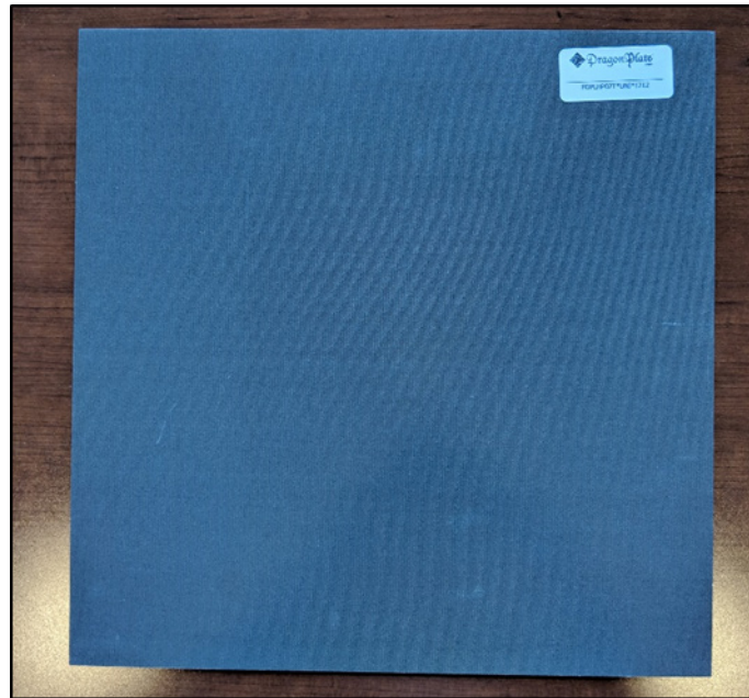
Figure 4. Unidirectional Carbon Fiber Plate (Manufacturer-Supplied)
