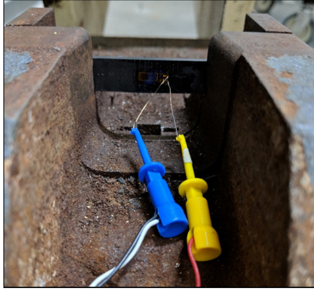
Figure 10. Example of Test-Ready Impact Specimen and Strain Gauge Wiring
