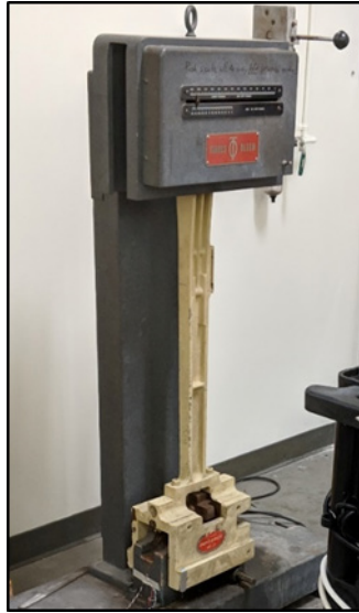
Figure 2. Charpy Impact Tester Used to Produce High Strain Rates
