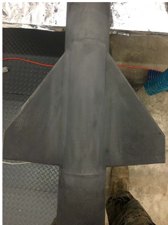
Figure 45. Sustainer Fin Can with Added Carbon Fiber Layer
