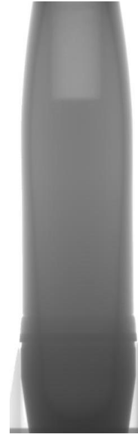
Figure 5: drilled with subcharge absent.
