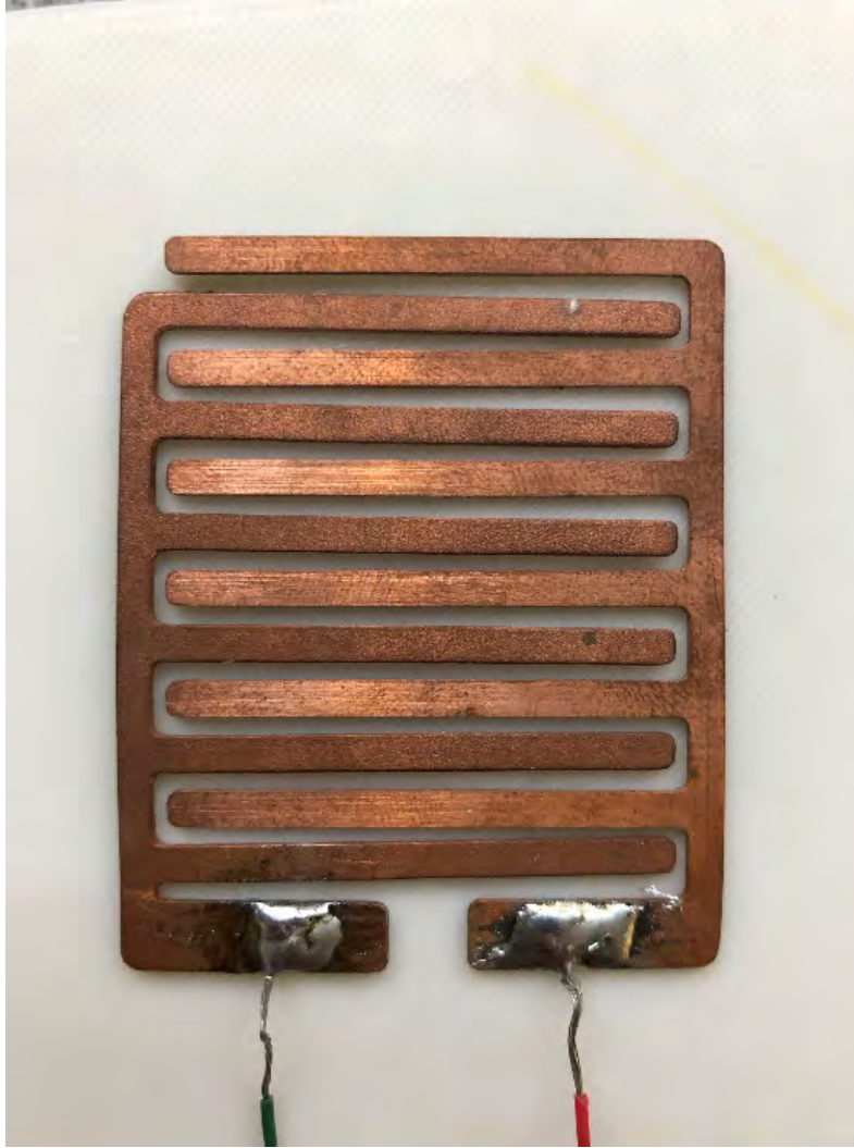
Figure 7. Copper Electrodes with Wires Soldered On
