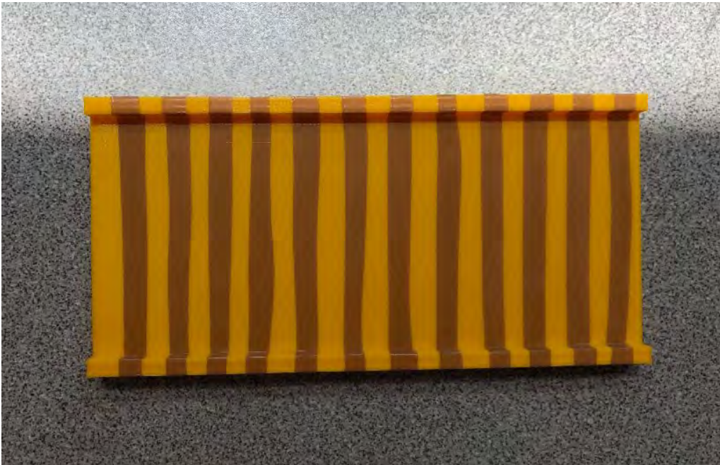
Figure 23. Track with Thin Adhesive PTFE Tape
