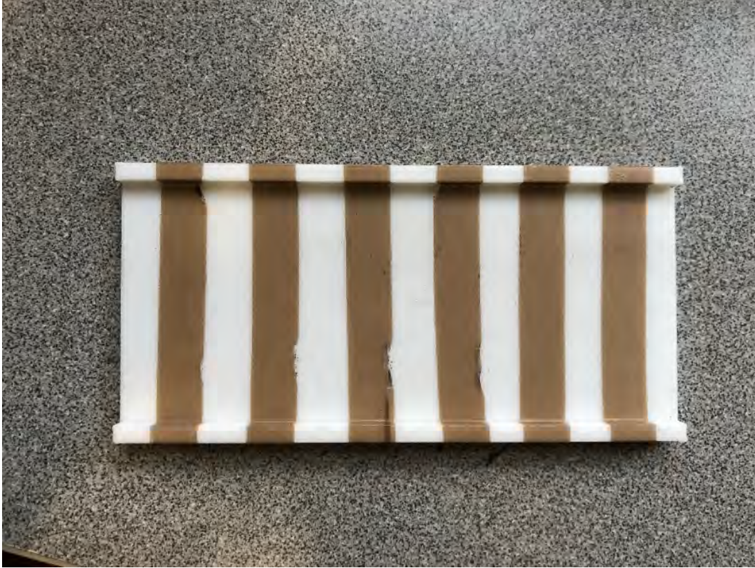
Figure 14. 3D Printed Final Track with Adhesive PTFE Tape
