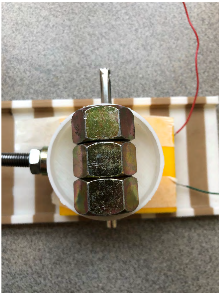
Figure 21. TENG Weight Holder with Three Bolts (96 grams)
