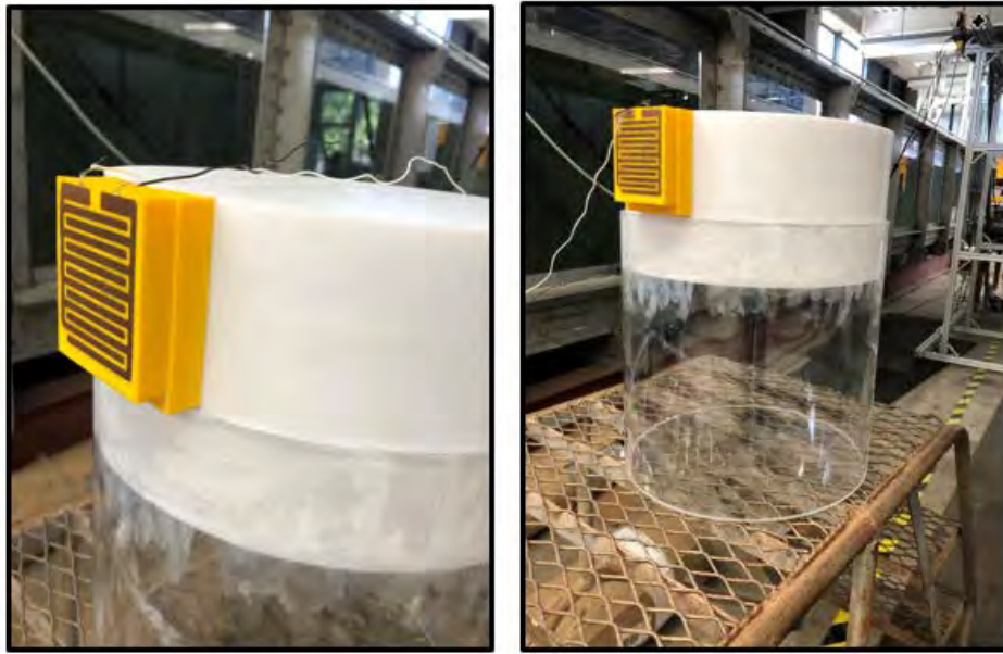
Figure 63. OC with TENG and Cap Attached, Close Up (left), Overall Experimental Test Article (right)
