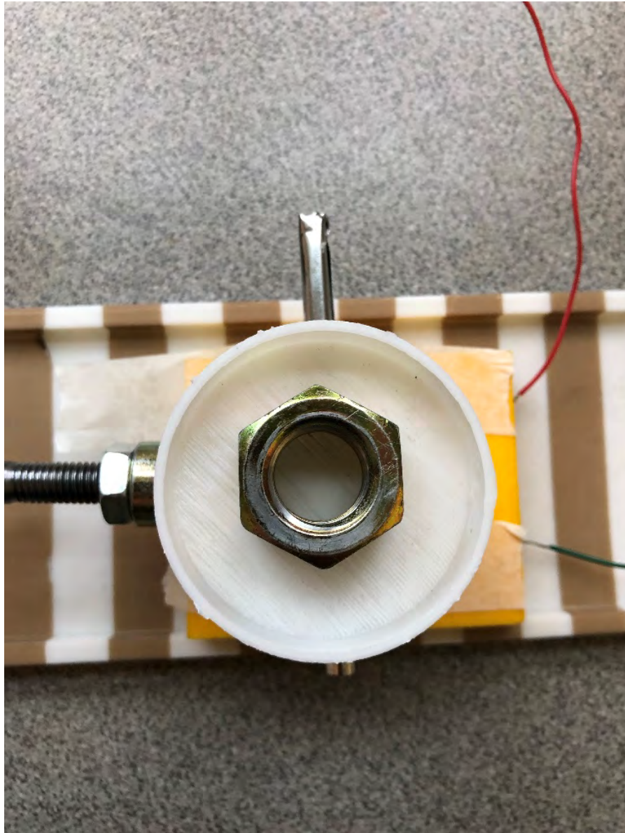
Figure 20. TENG Weight Holder with One Bolt (32 grams)
