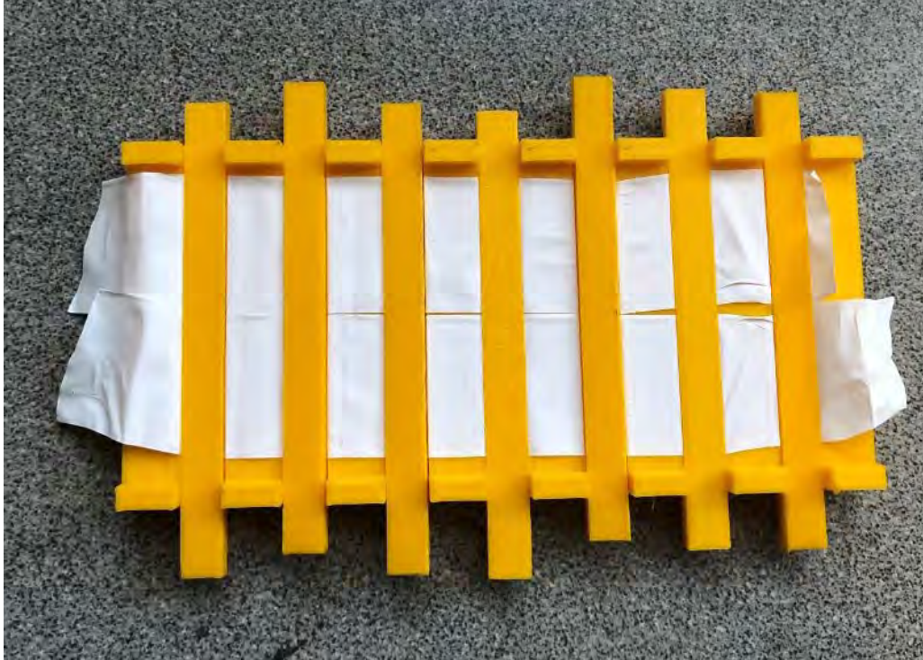
Figure 12. 3D Printed Second “Train Track” Track with PTFE Tape
