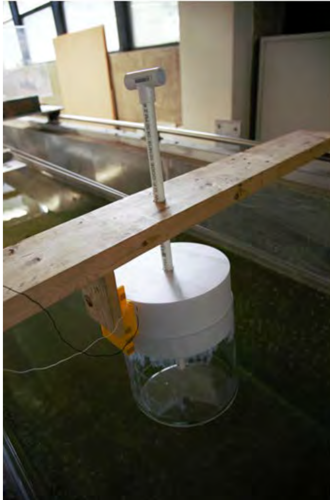
Figure 64. Full Setup of OC with TENG Attached in Wave Tank
