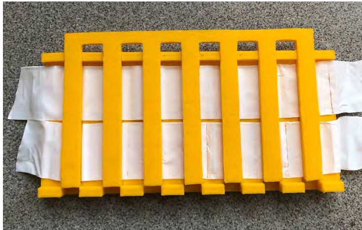
Figure 10. 3D Printed Original “Train Track” Track with PTFE Tape
