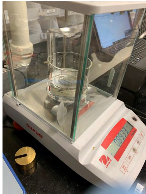
Figure 33. Nickel Sample in Ethanol Bath for Density Measurement
