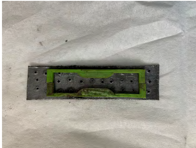
Figure 34. Mold to Produce Tensile Test Geometry
