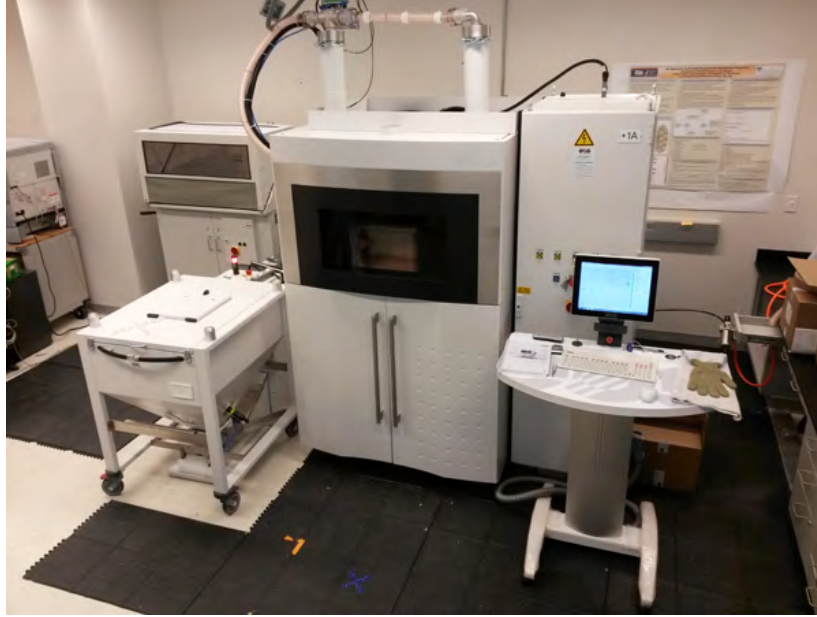
Figure 2. Powder Bed Fusion Printer. Source: [5].
