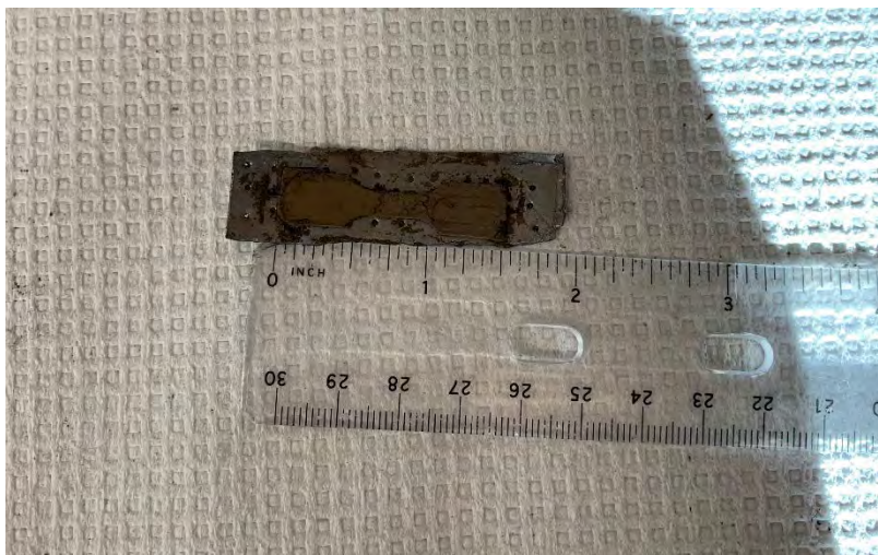
Figure 53. Iron Tensile Test Geometry Shape Before RES-SM Process
