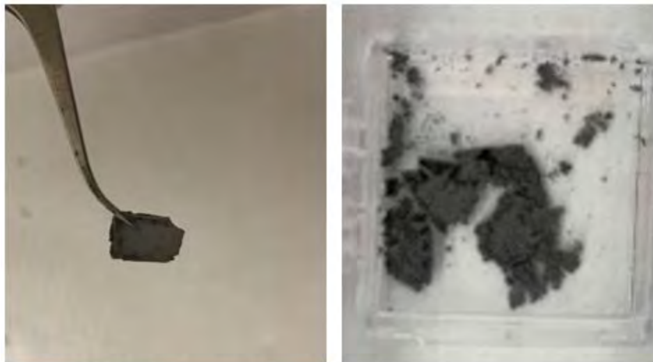
Figure 47. 10% FeO Iron Sample (left) and 50% FeO Iron Sample (right)
