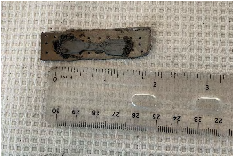
Figure 54. Iron Tensile Test Geometry Shape Before RES-SM Process
