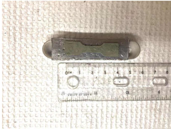
Figure 35. Pre-Bake Nickel Sample with the Mold Removed
