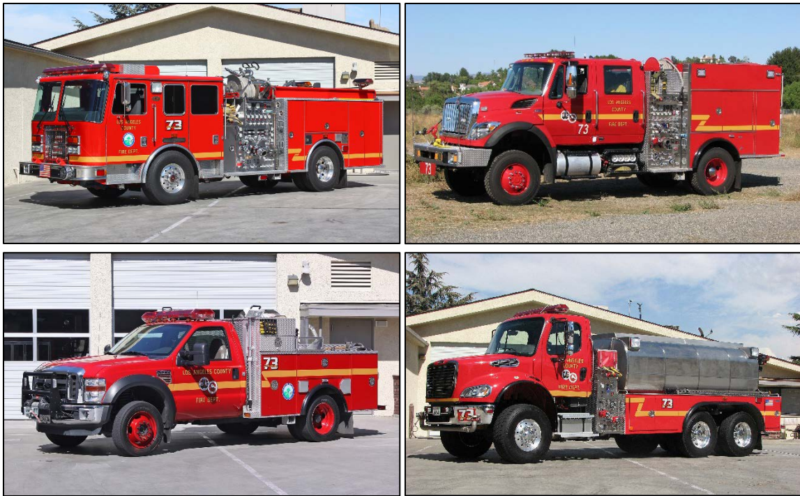
From left to right and top to bottom are the Type I, III, and VI engine variants, and the water tender. In respective order, images are sourced from: Johanson (2010a), Deyo (2011), Johanson, (2010b), and Johanson (2010c).
