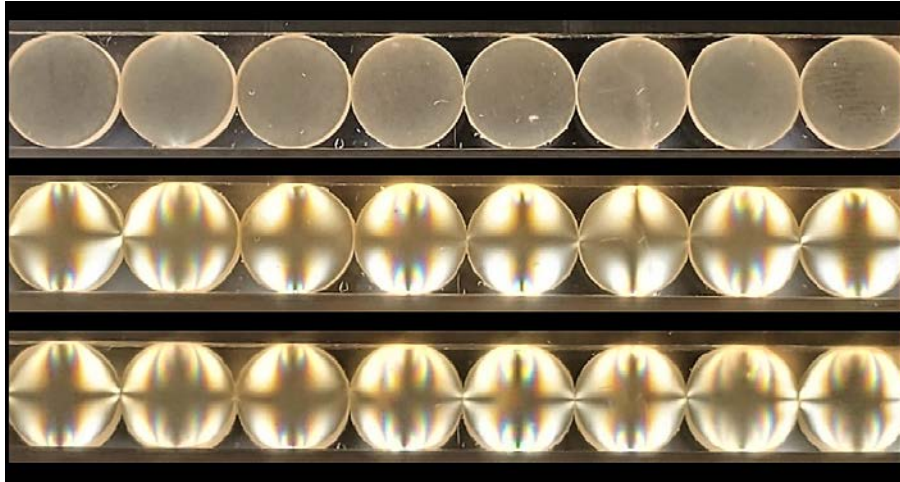
Figure 6. Image of photoelastic disks viewed using circular polarization
