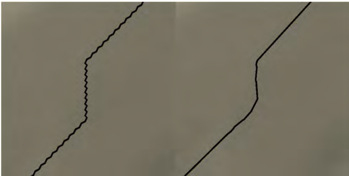
Figure 18. Visual Depiction of a Path Without Modifiers on the Left, and With a RaycastModifier Applied on the Right
