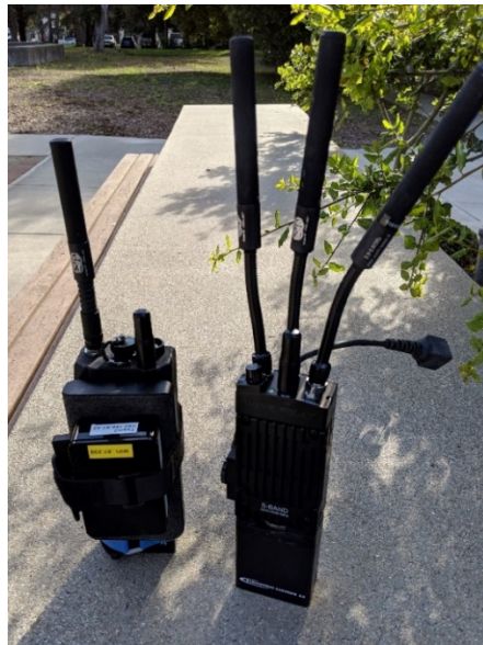
Figure 31. MPU4, SNMP Agent and Battery (left) and MPU5 (right) with the Corpsman
