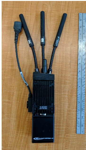
Figure 14. MPU5 with an Ethernet Connector and 3 RF Antennas
