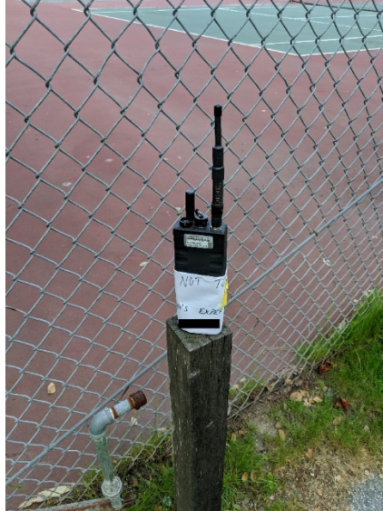
Figure 44. MPU4 Relay Node
