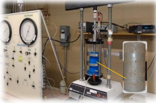
Triaxial soil compression test
