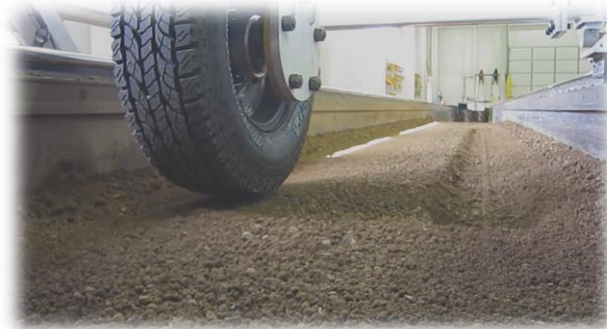
Single wheel soil bin mobility test at Caterpillar
