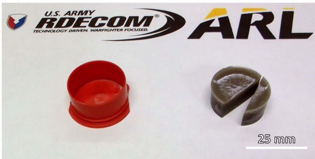
Fig. 2 Molding cup and produced sample with the sectioning line. The shown angle of the sectioning line is not representative of the aforementioned sectioning axis.
