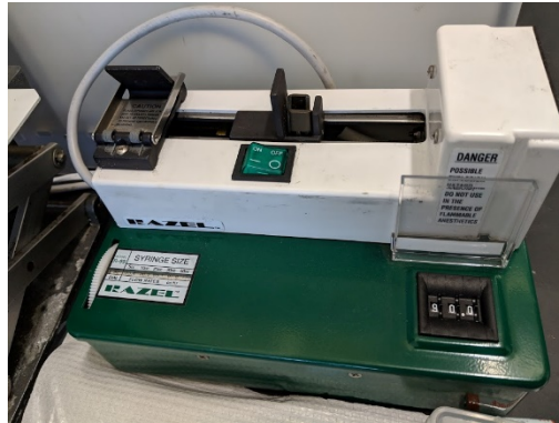
Figure 4. Syringe Pump (Razel R99-FM Syringe Pump)
