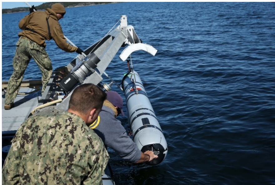
Figure 1. Sailors prepare to insert a UUV to search for underwater mines. Source: [1].
