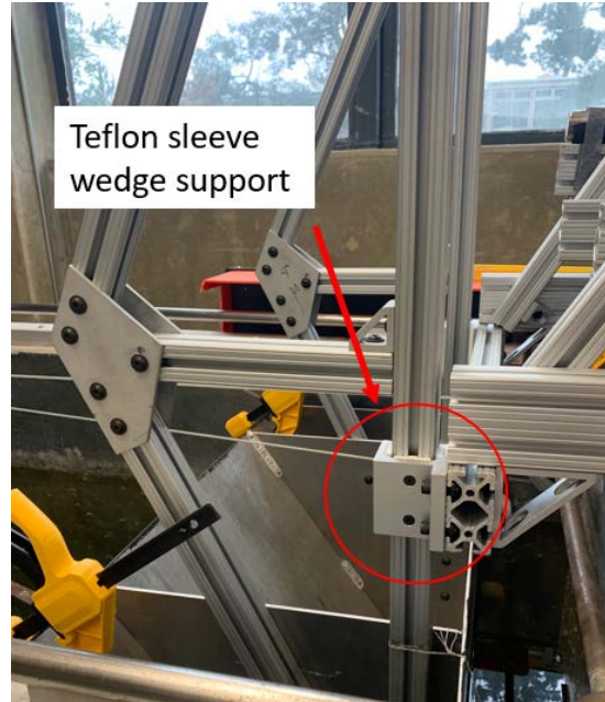
Figure 19. Current wedge support structure with Teflon sleeves
