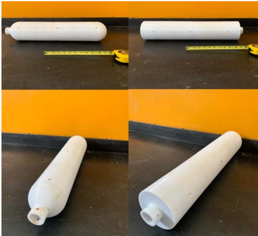
Figure 9. Model with hemispheric end caps and model with flat face end caps
