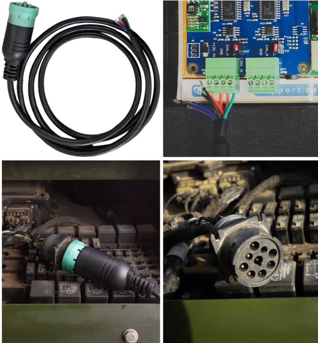
Top-left: 9-pin Deutsch J1939 connector cable. Top-right: wiring configuration of SAE connector wires to interface board CAN inputs. Bottom-left: physical connection of 9-Pin SAE connector to MTRV J1939 port. Bottom-right: exposed 9-pin Deutsch J1939 female connector on MTRV.
