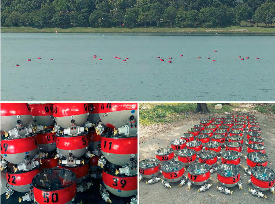
Figure 1-1: A small fleet of autonomous surface vehicles. Top panel: 25 buoys of a BoB system collectively operating at Bedok Reservoir, Singapore. Bottom left: Buoys stacked up during transportation to the field site. Bottom right: 48 buoys lined up before deployment [Zoss et al., 2018]
