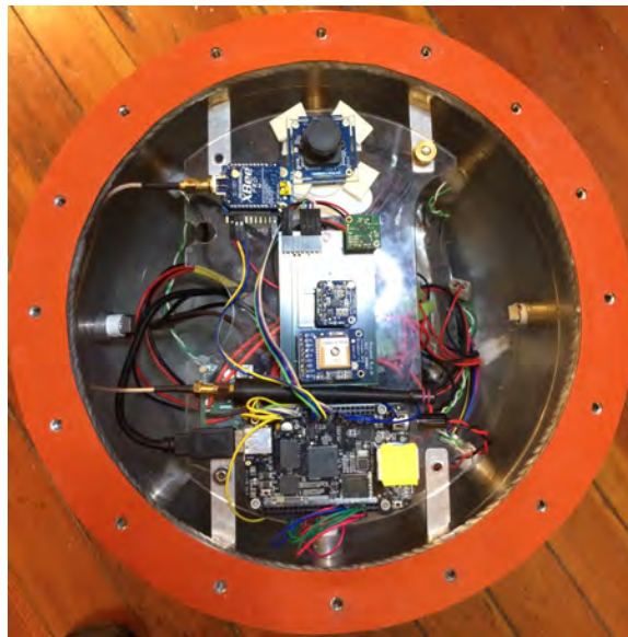
Figure 5-3: Location of the camera inside of the buoy, top center.
