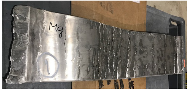
Fig. 34 Fracture of AZ31 after rolling
