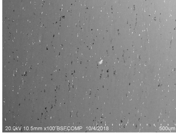
Fig. 4 Distribution of the particles in the original as-received material
