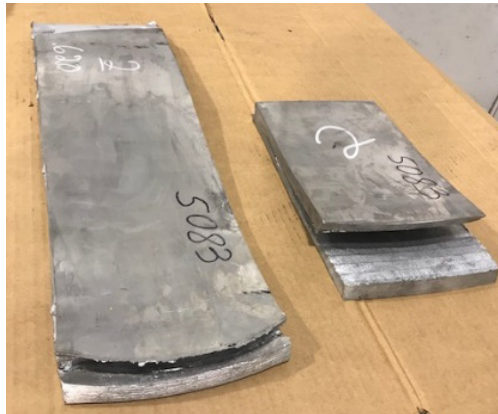
Fig. 31 Alligatoring of sample 2
