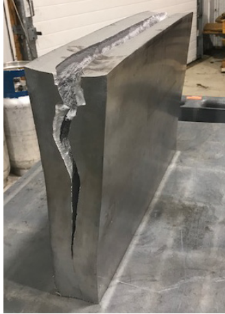
Fig. 30 Alligatoring of a full-scale large billet of AA5083 during rolling
