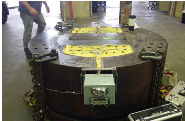
Fig. 26 The redesigned tool with the new DHS (without the covers in place; the thermal insulation and tops and electrical connections to the heater cartridges can be seen)
