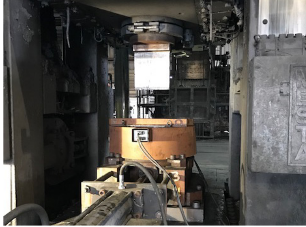
Fig. 28 Fully assembled large-scale ECAE die with the DHS at the 11,000-ton Ellwood press
