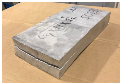
Fig. 32 Alligatoring of sample 3
