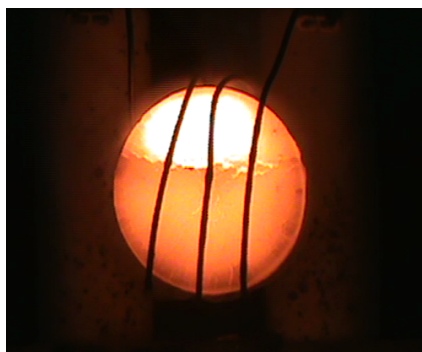
Figure 10. The Cobalt Sun: A Co(0)/LiClO 4 thermite disc (3 cm in diam.), after thermal ignition with an electrical resistor (wire) wrapped around it. (Still image captured from video 26 s after ignition: current to the wire is turned off and only part of the disc still glows white. The disc was glowing red for another 20 s.)
