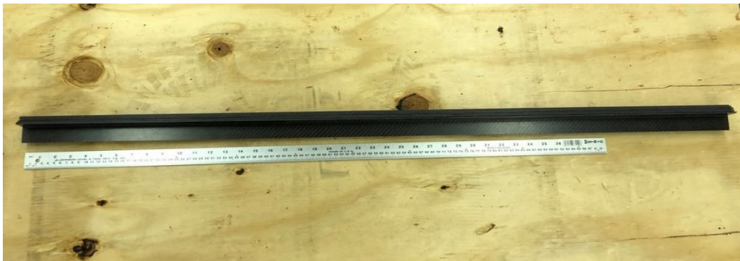
Figure 5. Carbon fiber bundle used in the test ( 8 \times 140 g angled carbon fiber and 2 \times 65 g).
