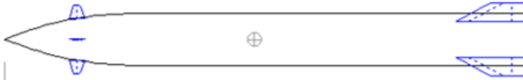
Fig. 4 Canard configuration of the AFF
