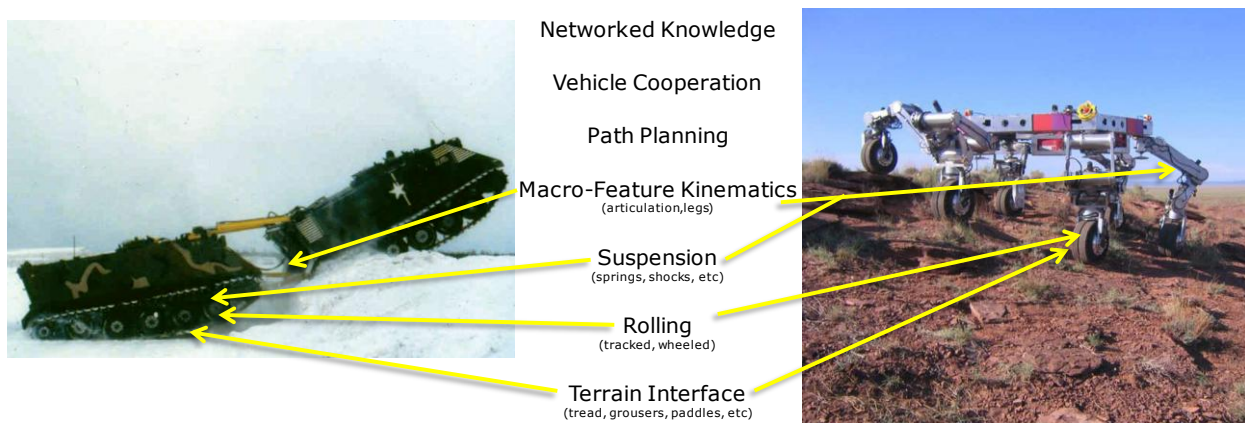
Figure 15. Fractal elements of mobility are length scale dependent. Moving beyond the physical ground-engagement space you enter the pure cognitive space (path planning, cooperation, and networked knowledge).
