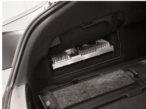
Figure 24. Audi's zFAS central driving system is based on the nVidia Tegra K1 GPU with 192 cores.
