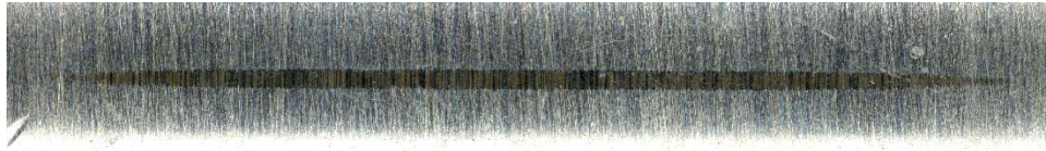
Figure 20. F-24 showing a 5.8mm x 133 micron wear scar
