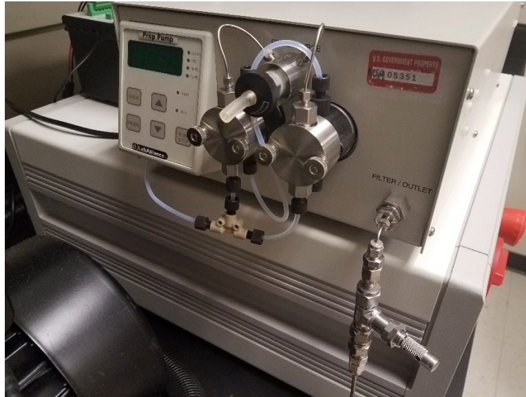
Figure 8. Pump added for test fluid flow rate control
