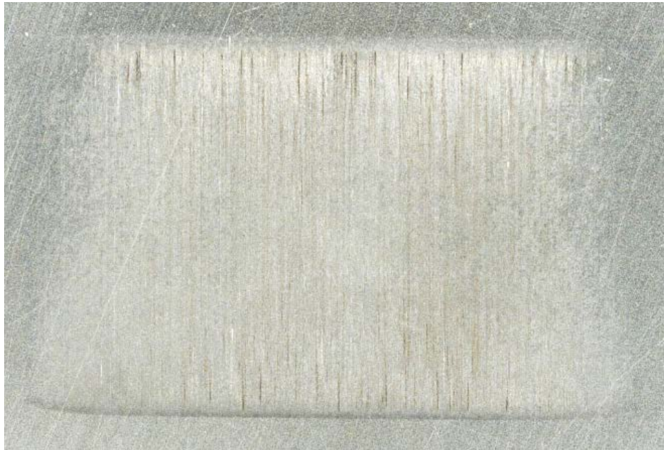
Figure 19. FT-SPK wear marks on the disk
