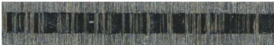
Figure 25: ATJ w/ 8ppm CI/LI showing 169 micron wear scar
