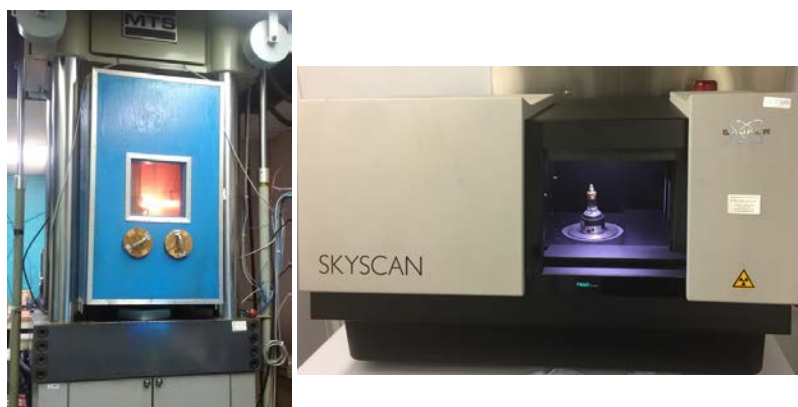
Figure 2. Testing stages used in compaction experiments. Left , the CRREL MTS stage with environmental chamber, and right , in situ testing stage within the micro-CT scanning chamber.
