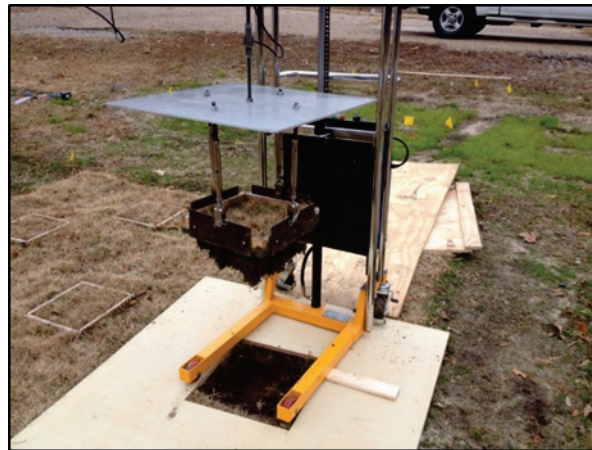
Figure 9. Sod pull-box system with tensiometer in use in the pilot demonstration.
