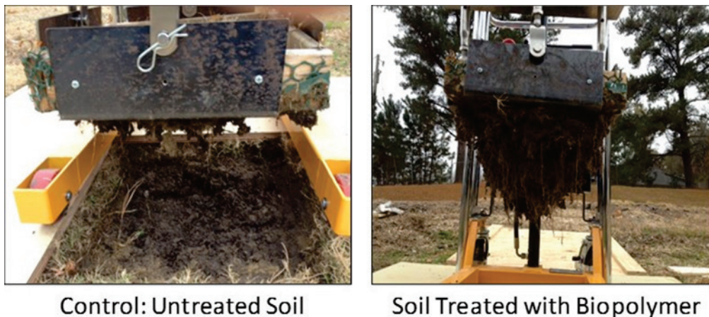
Figure 12. Comparison of root development in overwintered Bermuda grass sod when left untreated (Control – left) or treated with biopolymer (right).
