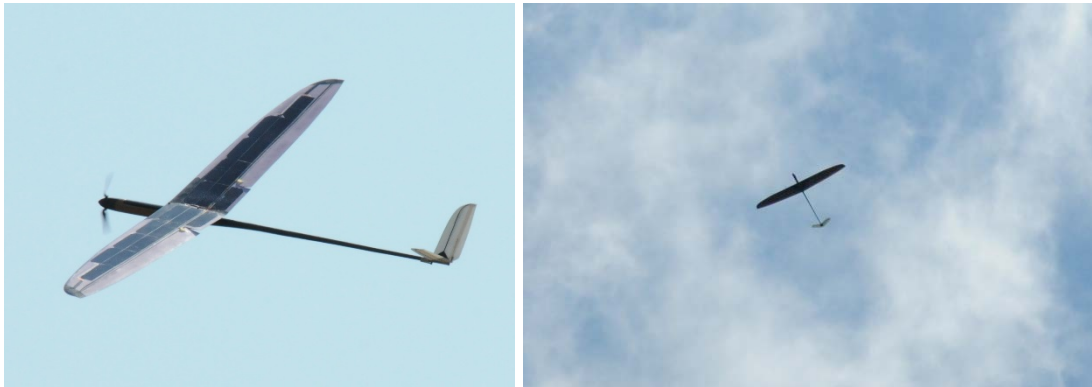
Fig. 1—NRL’s Solar Aurora showing the wing-integrated solar array (left) and at altitude while soaring (right)
