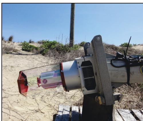
Figure 2-7. Lidar scanner, housing, and mounting plate connected to mast.
