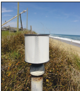
Figure 2-4. Reflector used to rectify lidar scan data.
