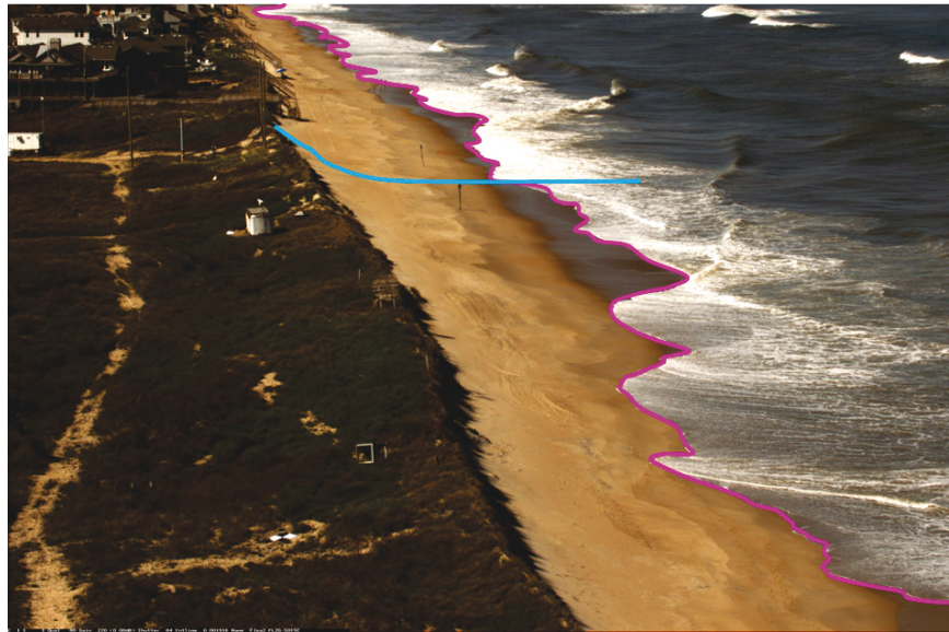
Figure 4-12. The cross-shore position of wave runup (magenta) along the beach at a single point in time from Argus video imagery. The blue line represents a single cross-shore profile through time.
