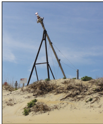
Figure 2-6. Lidar mast and scanner supported by cradle over dune crest.
