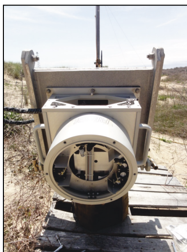
Figure 2-8. Image of mounting plate to which the lidar is attached.
