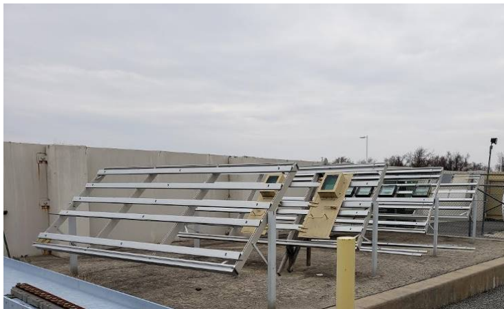
Fig. 4 Outdoor exposure racks at Aberdeen Proving Ground facing south
