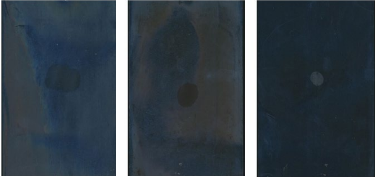
Fig. 7 Oxalic acid test results on Class 1 black oxide. From left to right: chromic acid seal, Bonderite M-CR 5900, and SurTec 555.
