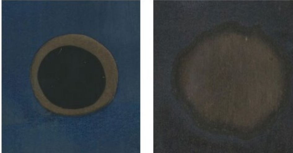
Fig. 1 Passing oxalic acid test (left) and failed oxalic test (right)
