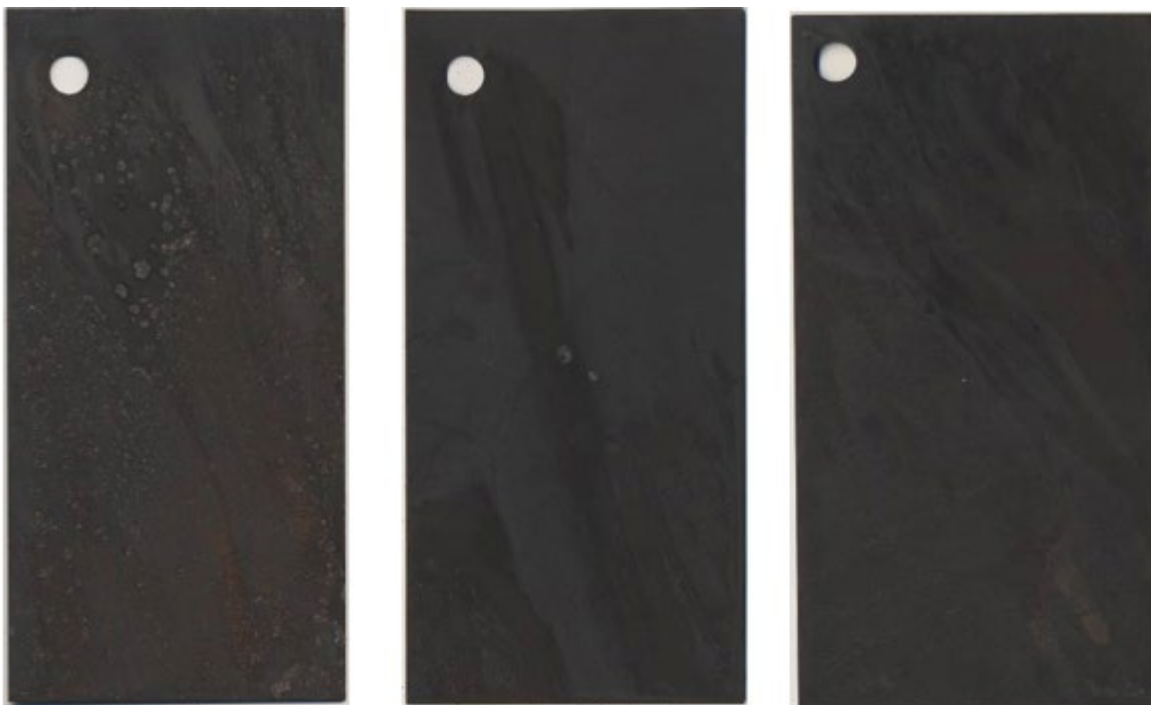
Fig. 9 Humidity test results for Class 4 black oxide, with supplementary preservative. From left to right: chromic acid seal, Bonderite M-CR 5900, and SurTec 555.
