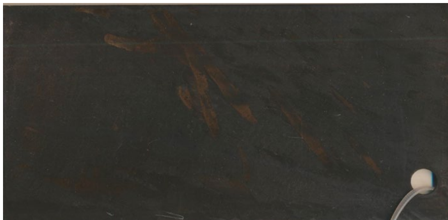
Fig. 13 Class 4 panel without supplementary preservative with flash rust that occurred in ambient laboratory environment
