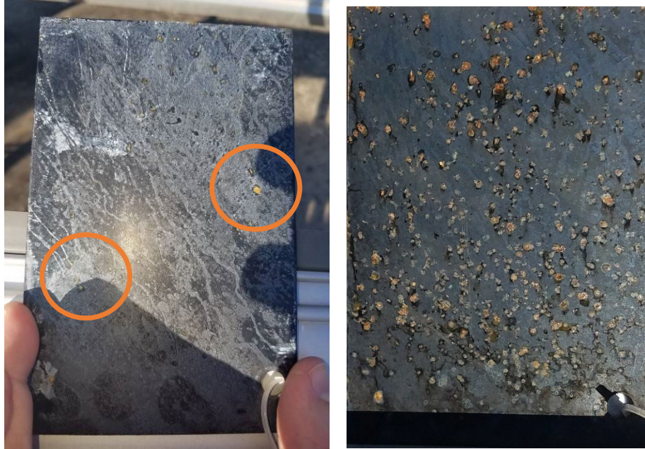
Fig. 14 Chrome seal after 1008 h of outdoor exposure (left, with supplementary preservative; right, without supplementary preservative)
