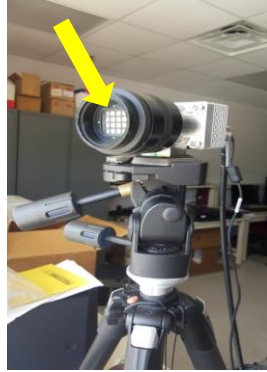
Figure 1. Photograph of the SOC716-VNIR camera shows the spectral filters in their 4x4 matrix holder.
