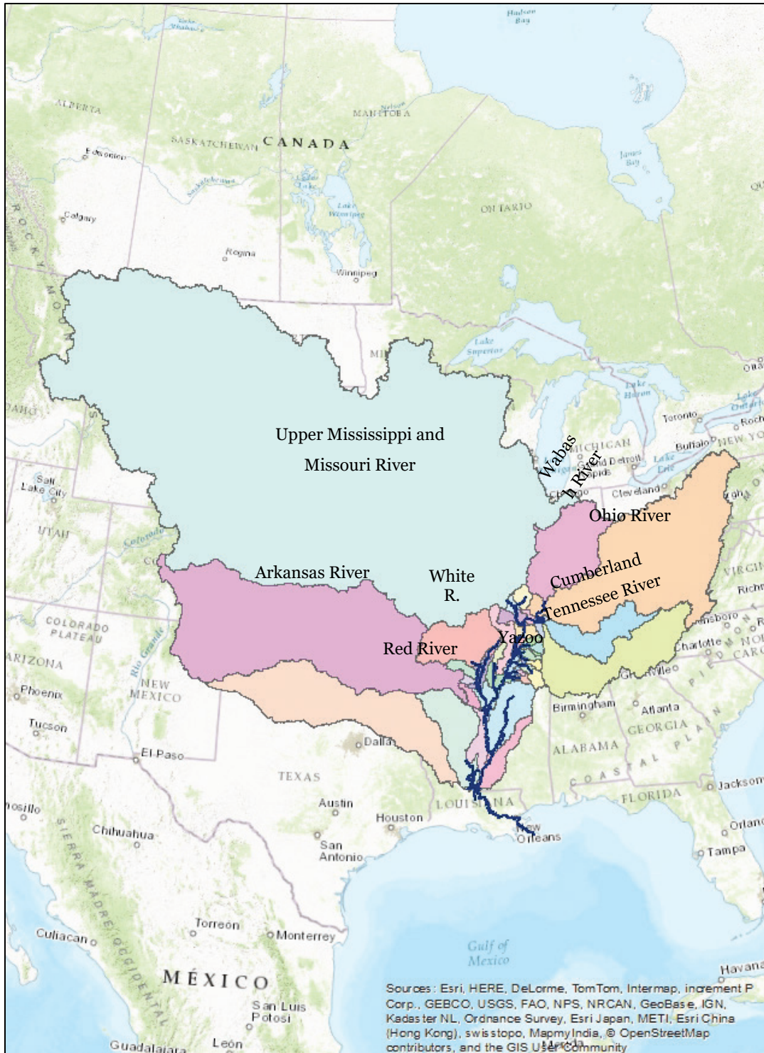
Figure 3-1. Hydrologic connections of the HEC-RAS model.
