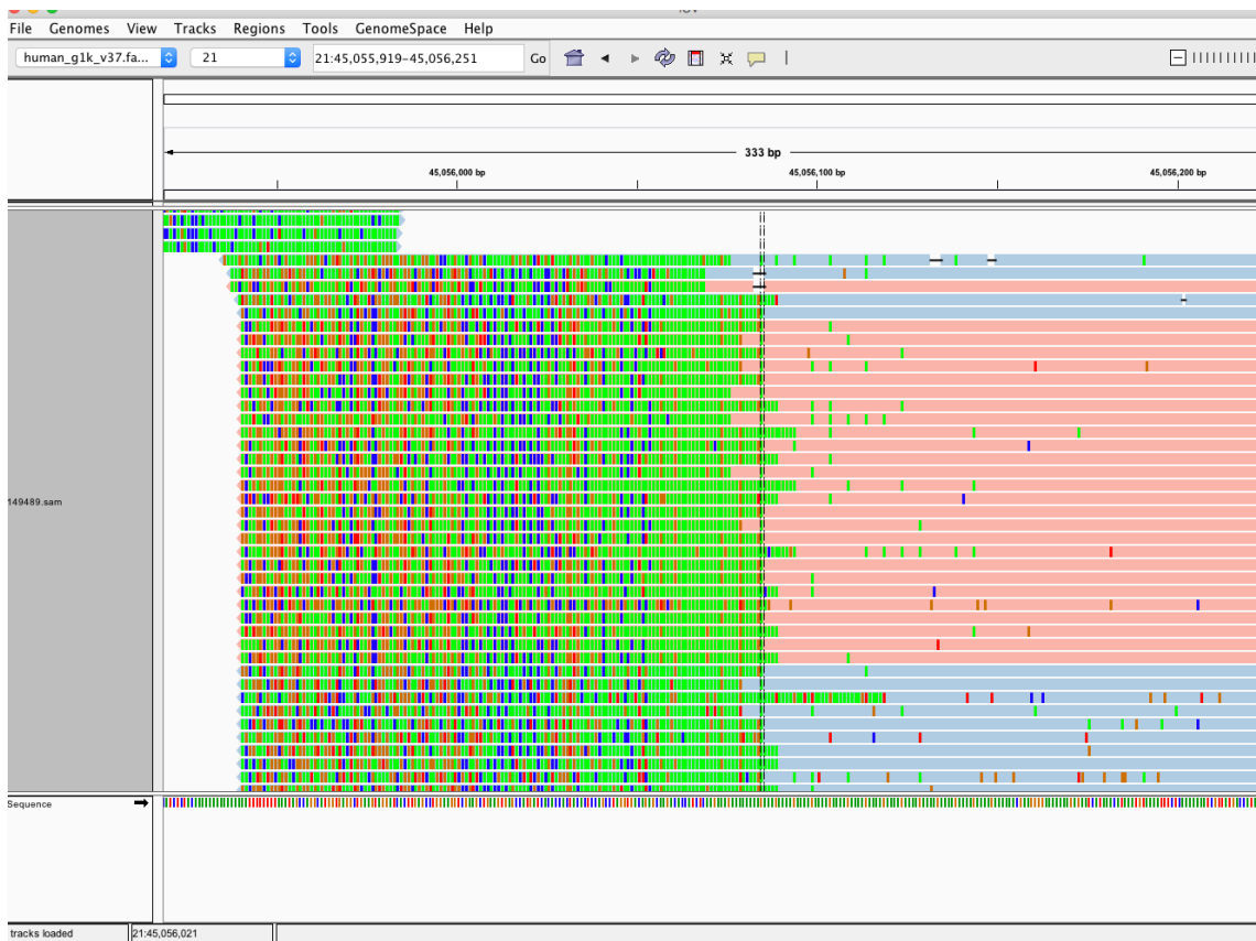
Fig. 12. Read failures at PentaD locus. Integrated Genome Viewer screenshot of a single molecular barcode family that becomes highly error prone after exiting the PentaD STR. Each read is derived from a single cluster on the sequencer. Data suggest that the sequencer itself is having difficulty properly sequencing the STR.
