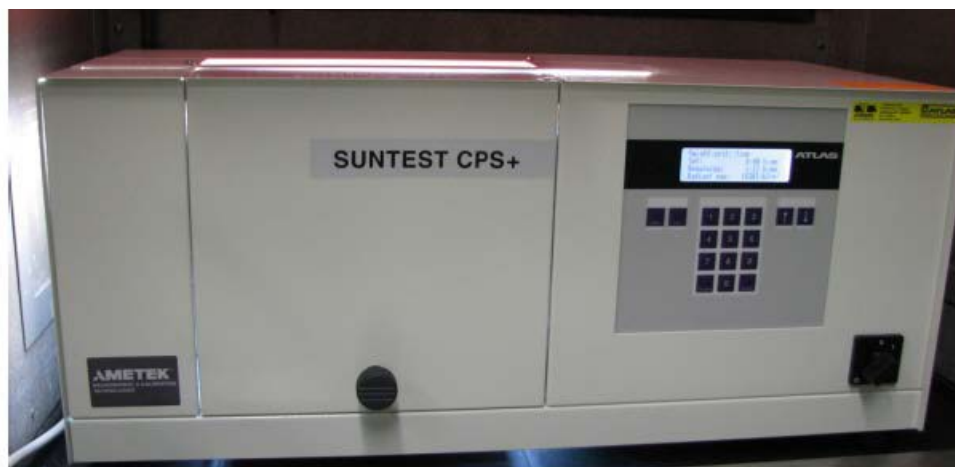
Fig. 1 Suntest CPS+ xenon test instrument used to evaluate photolysis of PrNQ in aqueous solution
