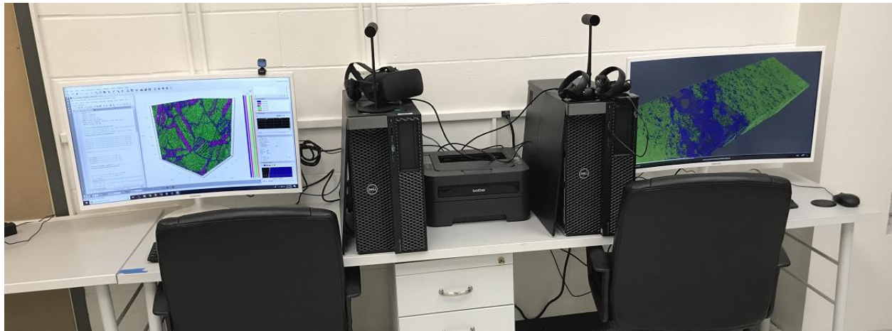
Figure 1: Two Dell 7920 Precision workstations showing the VR headsets and the ARIVIS InViewR and Vision 4D Software.
