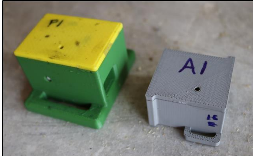
Figure 3: First (3.0 in 3 ) and second (0.7 in 3 ) generation mTBI sensing systems, housing all electronics and sensors. A 75% volume reduction was achieved through improved packaging and reduced system complexity, which enabled higher numbers of overpressure field test units
