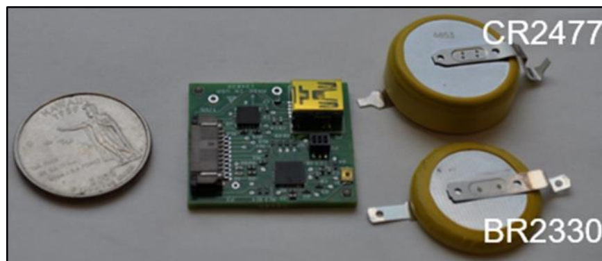
Figure 34: Two batteries traded during prototyping, with US quarter for scale. CR2477 was selected to maximize system battery life.
