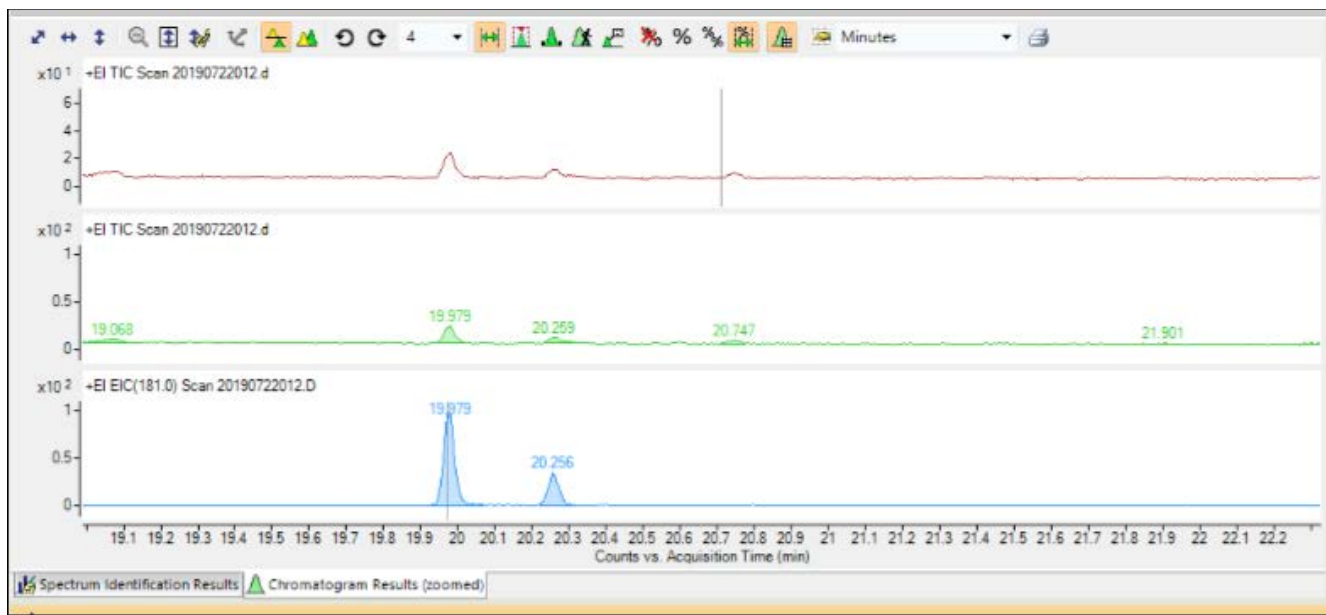
Figure 9: Acrolein oxime chromatogram on Agilent GCMS showing both enantiomers (20.0' and 20.3').
