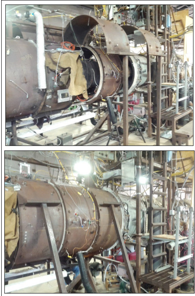
Figure L-2. Nacelle test fixture (top) interior view showing location of spray fire and closed configuration in preparation for testing (bottom).
