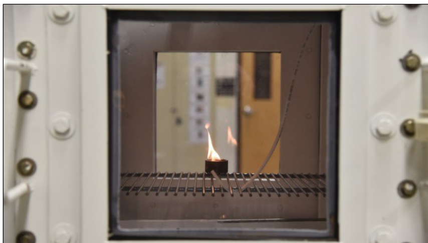
Figure 2.4-2. The 8-ft 3 test chamber employed in by-product testing.
