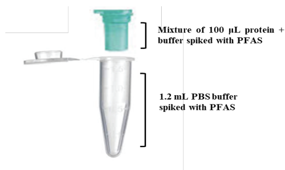
Figure 1. The schematic of equilibrium dialysis experiment
