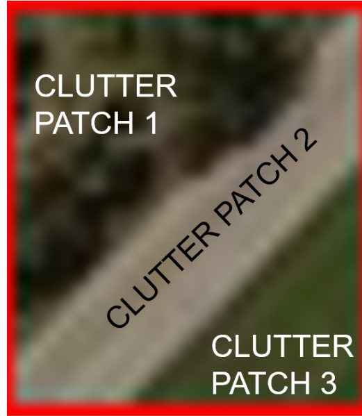
(b) This resolution cell contains three clutter types: foliage/trees (patch 1), concrete (patch 2), and grass (patch 3). This thesis concerns scenes with resolution cells that contain multiple clutter patches. The overall distribution for the radar signal return from this cell is a convolution of the three individual clutter patch distributions relative to their areas.
