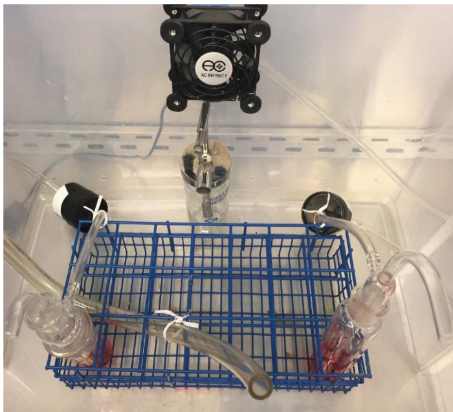
Figure 13: Top View of ATC Set-up for Impinger/STA Comparison. Red Impinger Fluid Added for Illustrative Purposes
