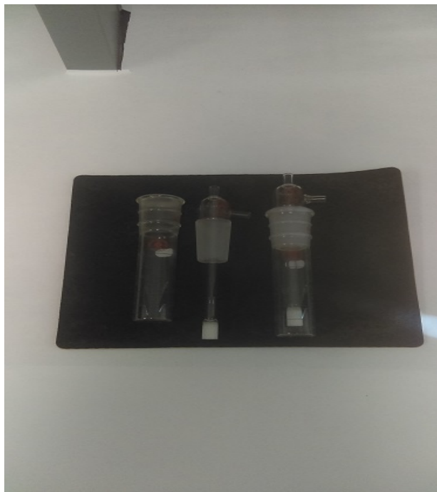
Figure 15: Fritted Glass Bubbler Components and Assembled Device
