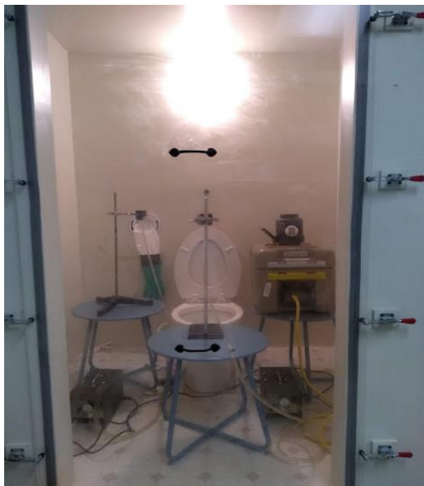
Figure 19: LAC with Toilet and Air Samplers Installed
