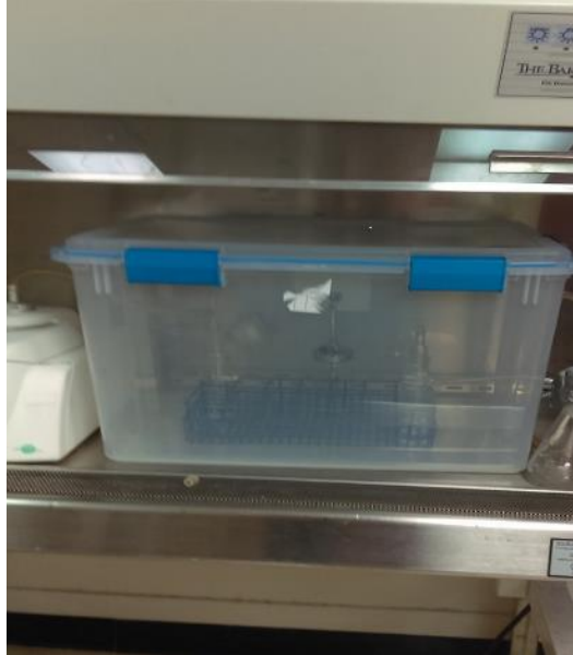
Figure 4: Aerosol Test Chamber in Biological Safety Cabinet
