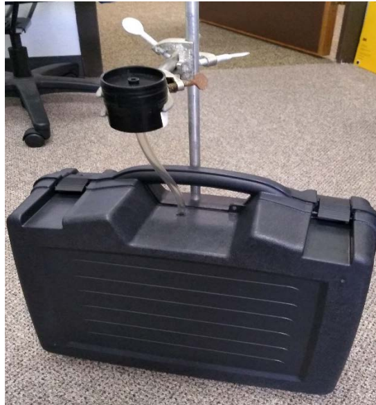
Figure 31: MCE Filter with Pump in Noise Dampening Enclosure
