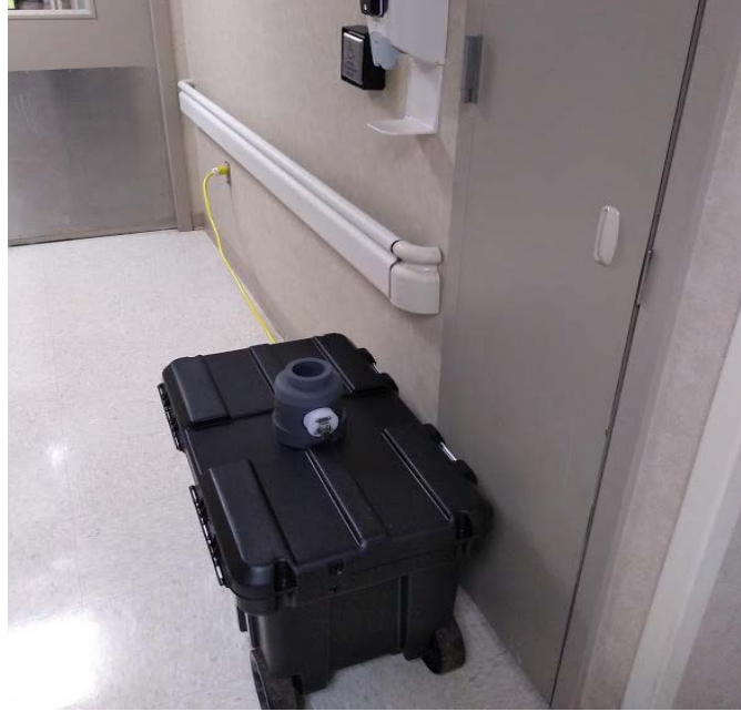
Figure 32: DFU-1000 in Noise Reducing Enclosure
