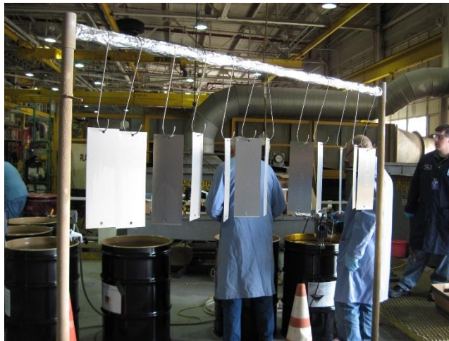
Fig. 9 Panels drying on portable rack after zirconium treatment at LEAD
