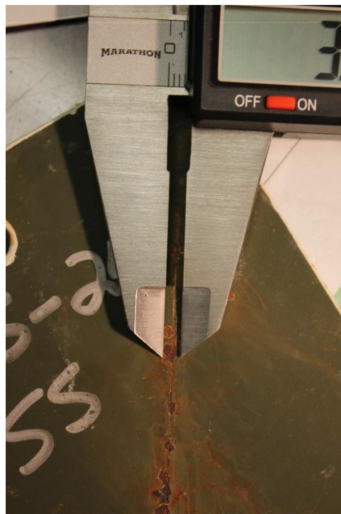
Fig. B-1 Measuring scribe creep with calipers
