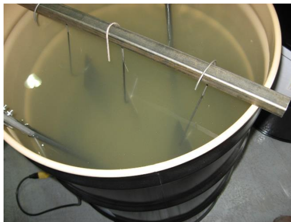
Fig. 8 Panels in cleaner tank at LEAD demonstration
