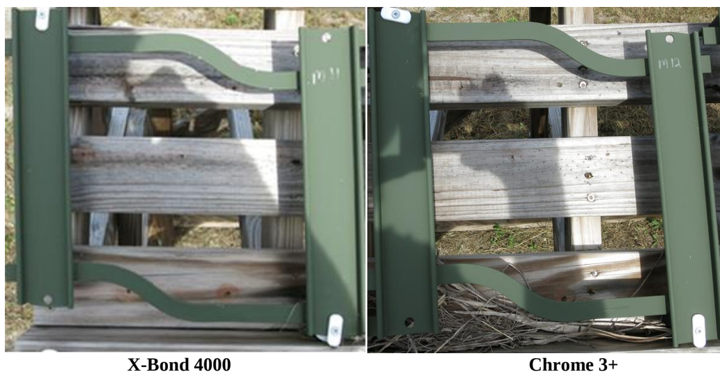
Fig. 42 CCAFS 24 months' exposure from December 2014 to December 2016 of aluminum HMMWV battery hold-down brackets treated with chrome 3+ vs. X-Bond 4000 coated with MIL-DTL-53030 primer and MIL-DTL-64159 topcoat
