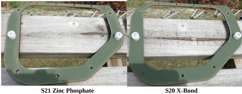
Fig. 43 CCAFS 24 months' exposure from December 2014 to December 2016. CRS lift hook D-ring surrounds treated with X-Bond vs. zinc-phosphate and painted with MIL-DTL-53030 primer and MIL-DTL-64159 topcoat at MDMC-PPA.
