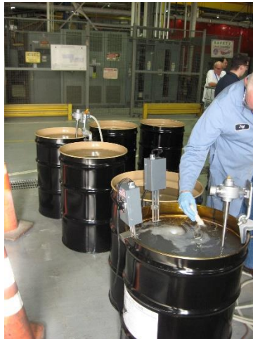
Fig. 6 Setup of the X-Bond cleaning and treatment process at LEAD
