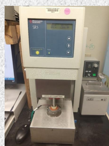
Figure 9. Rheometer test setup
