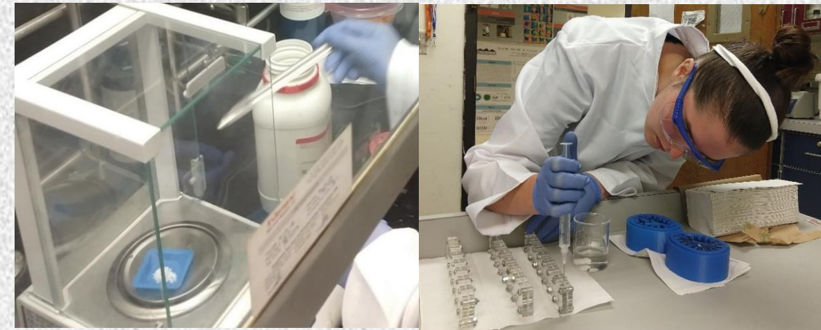
Figure 6. Student synthesizing PAA (left) and filling disk molds with PAA solution (right)
