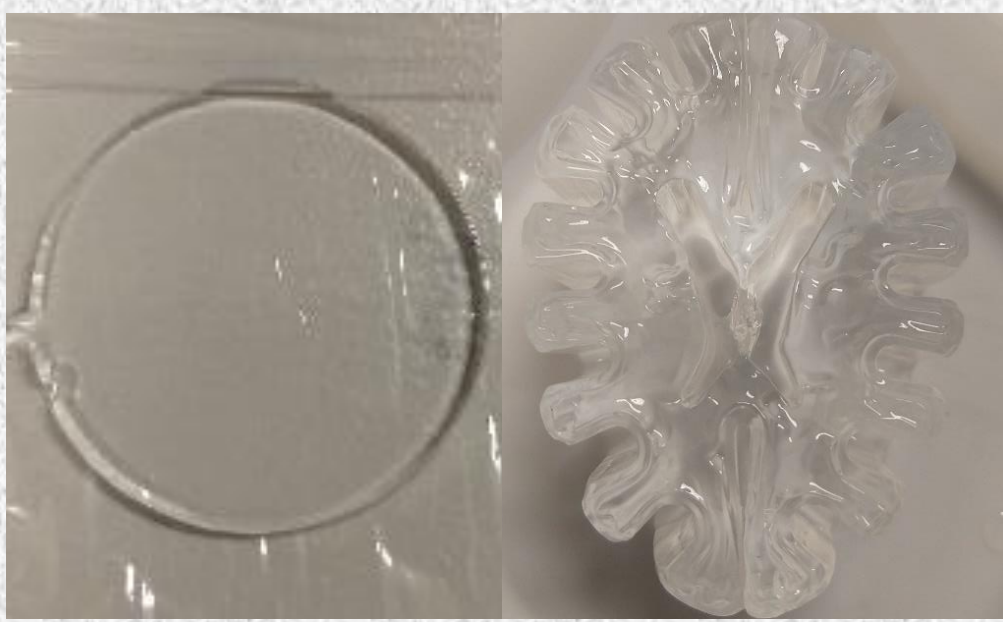
Figure 7. PAA disk samples swelled for 36 hours (left) and miniature brain mimics swelled for 3 days (right)
