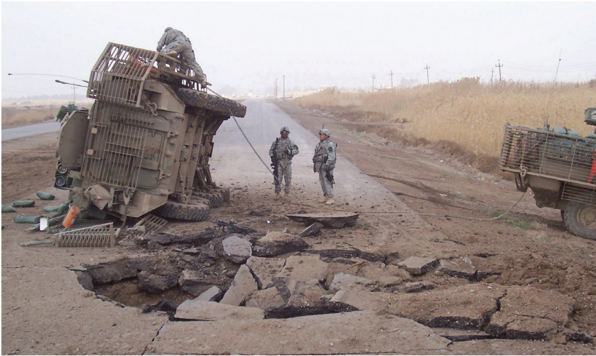
Figure 3.11 Stryker After an IED Blast in Afghanistan
