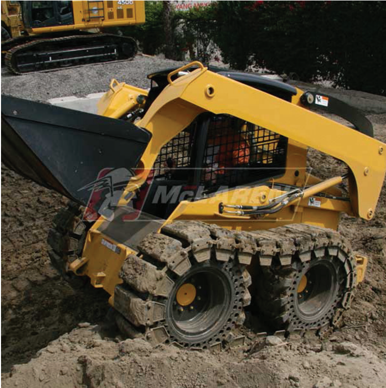
Figure 4.2 Illustration of Tracks Over Wheels for Forest Machines and Construction Vehicles
