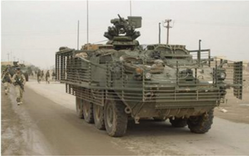
Figure 3.8 Stryker Infantry Carrier in Iraq Fitted with Slat Armour
