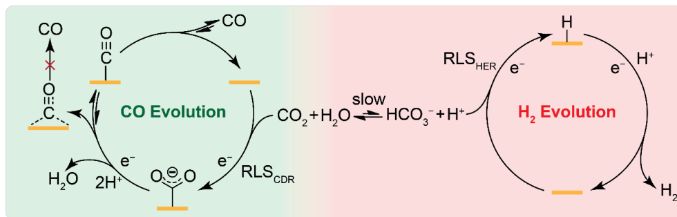
Figure 2 – Predictive mechanistic model constructed for the mechanism for CO (green) and \text{H}_2 evolution (red) occurring simultaneously on Au electrocatalyst surfaces during \text{CO}_2 reduction.
