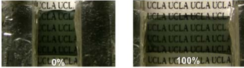
Figure 6. Schematic illustration of a PTB7:PC 71 BM:DIO blend film upon reversible stretching and relaxation.
