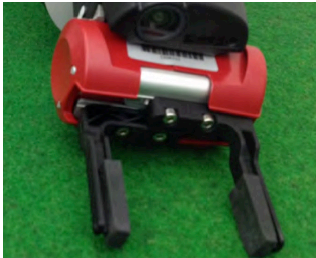
Figure 10: The end of a Baxter arm includes a RGB camera, an infra-red sensor, and grippers.
