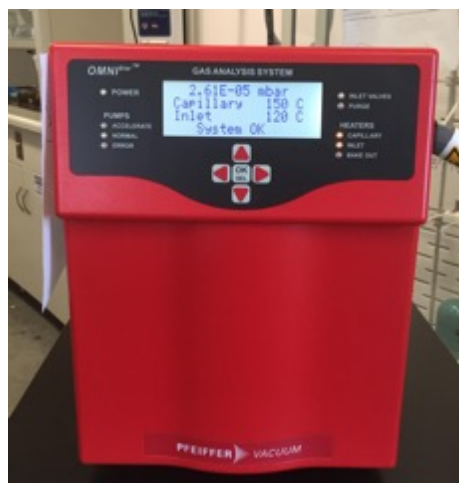
Figure 2 Pfeiffer OmniStar GSD gas analyzer as-installed in PI Hicks' laboratory.
