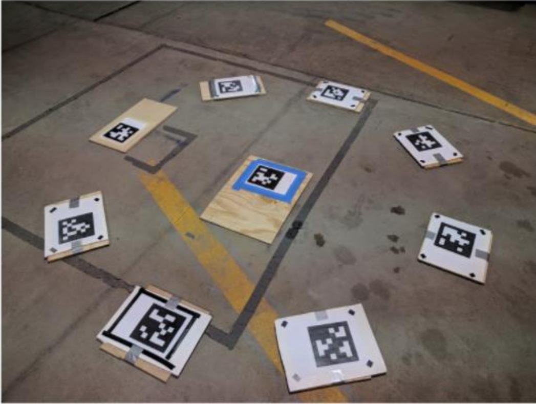
5: April Tags laid out for testing in a circle of radius 2m
