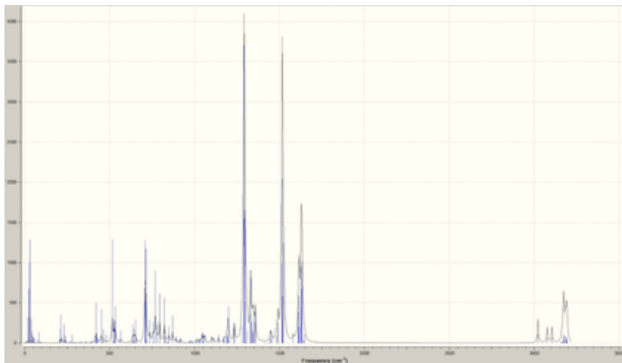
Figure 24. DFT calculated IR spectrum (arbitrary units) of dye FH94931, C_{38}H_{32}N_2 , in solvent Acetone.
