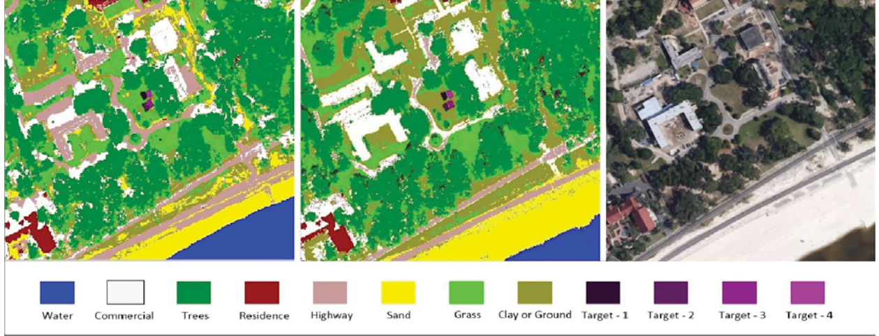
Figure 14: Gulfport dataset: CNN using HSI data only (left) and fused HSI and LiDAR data (middle). Google map view (right). Classes labeled Targets 1-4 correspond to materials placed on the ground, on elevated tables, and under trees by the NGA.
