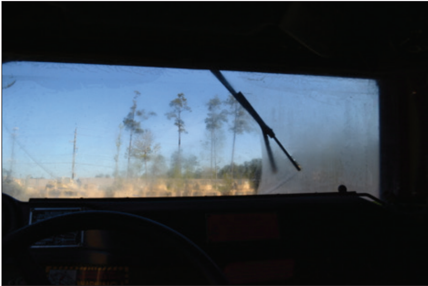
Figure 1.3 Interior View Through a Delaminated Windshield
