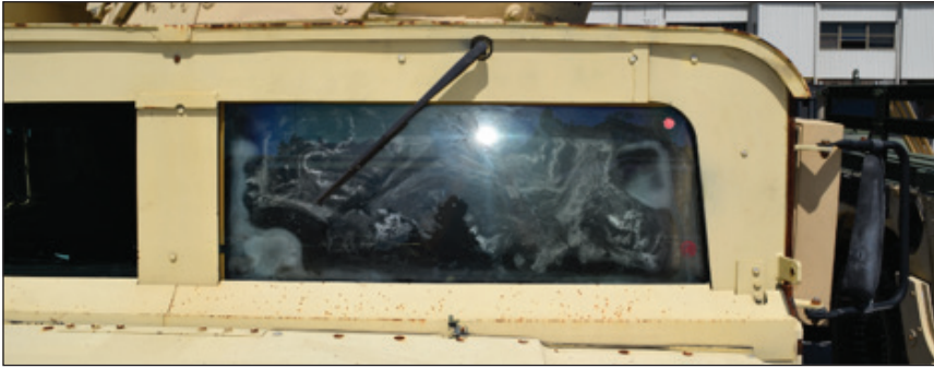
Figure 1.2 Example of a Delaminated Windshield
