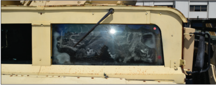
Figure S.1 Example of a Delaminated Windshield
