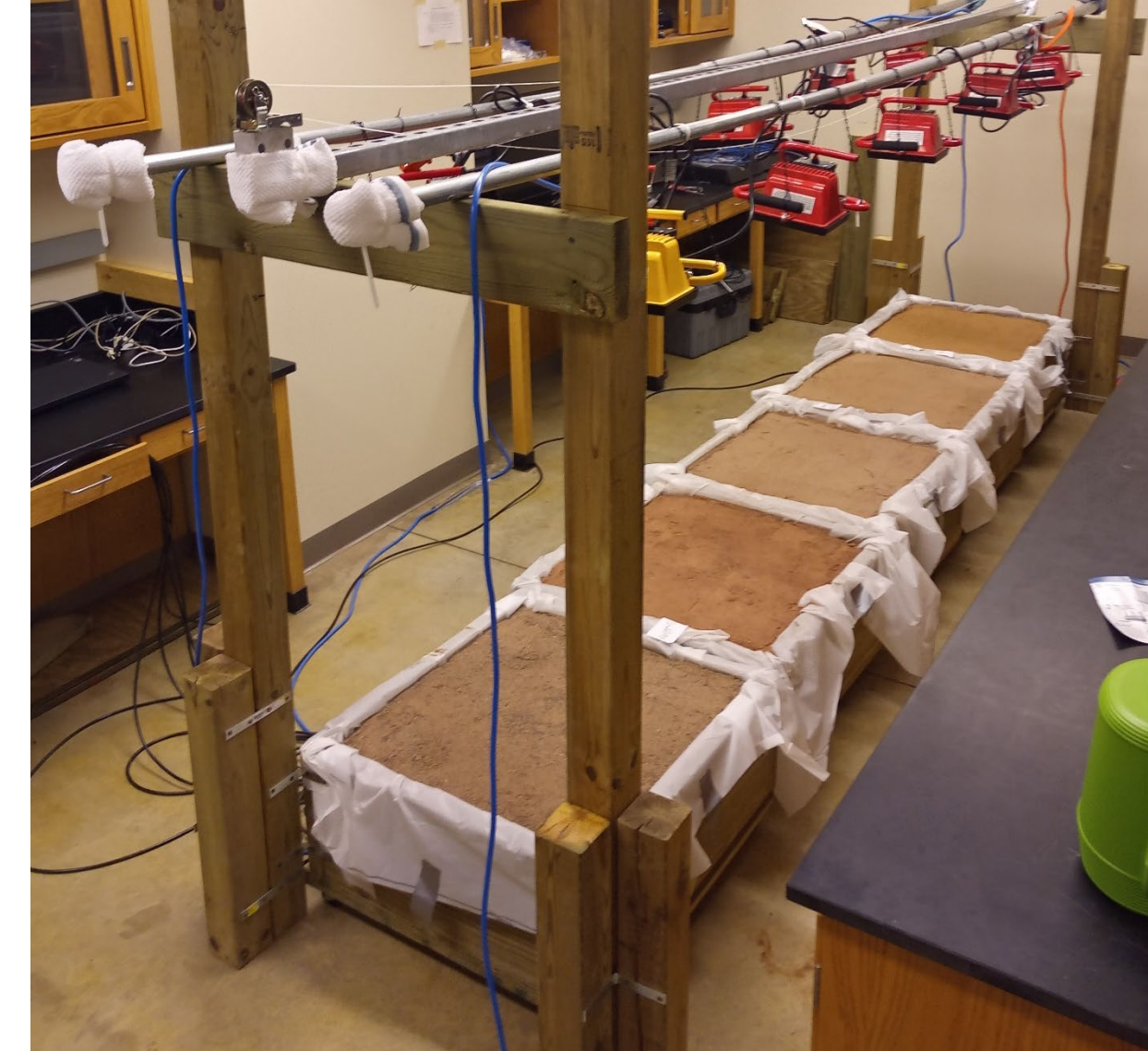
Figure 4. Shows the lab setup of the 5 KRC soils. The soils in order from bottom left to top right: 2NS, Stability, Rink, Coarse, and Fine. Above each bin are two 500-Watt work lights, and the middle bar is the track the hyperspectral camera is moved along.
